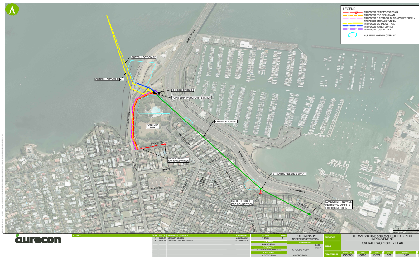
Figure 3 Engineering Outline Plan showing Outfall Option A
