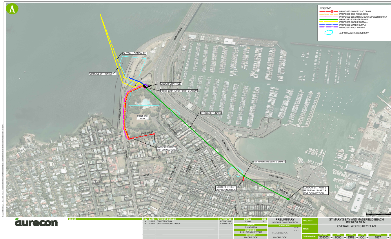
Figure 3 Engineering Outline Plan showing Outfall Option A
